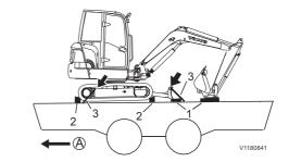
Tying down on small trailer (3.5 t) (Use anti-slide mat for steel tracks) A: Driving direction
