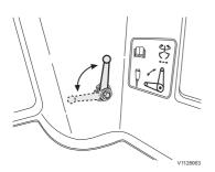
The shut off valve is located in the cabin on the right hand side close to the floor mat.
