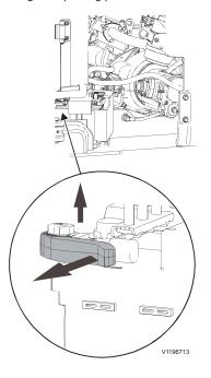
Battery Quick connector under left hood
