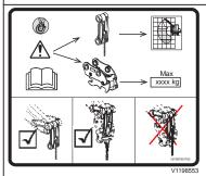
15 Lifting with a Quick Coupler (if installedt).
