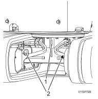
Towing eye (1) on lower frame The outer eyelets (2) are not suitable for towing or tying down.
