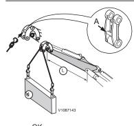
The blade must be in upper position during lifting operation if no hydraulic safety valve is installed.
